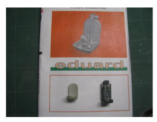
The Cockpit: The seat to the lower left is what Tamiya includes and is not correct. Maybe for test flying the prototypes but not production. After searching my personal library of books to view the correct seat I found this Eduard seat on Ebay and is accurate for the early Navy production aircraft. It has nicely molded seatbelts as well.
