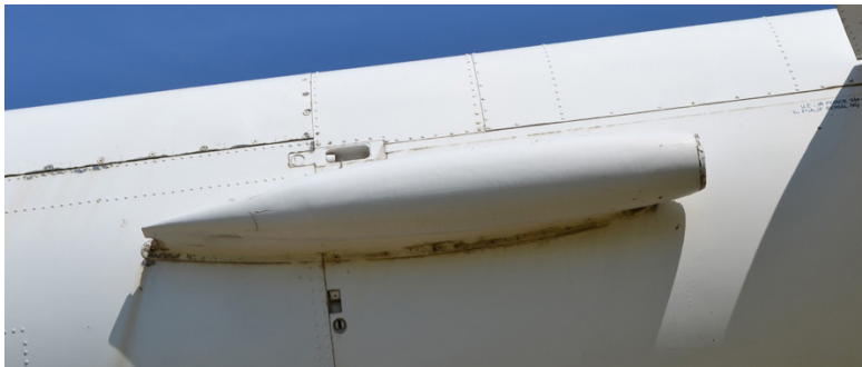
Close up of right-side air scoop. This scoop is on the right side only.
