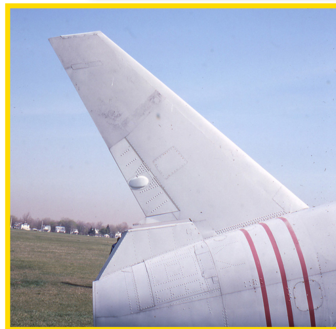
Aft fuselage and rudder of the Snark at the National Museum of the USAF. Note the “parachute container” has a sloped aft surface and is not squared off as is the Hill example in photo 8.
