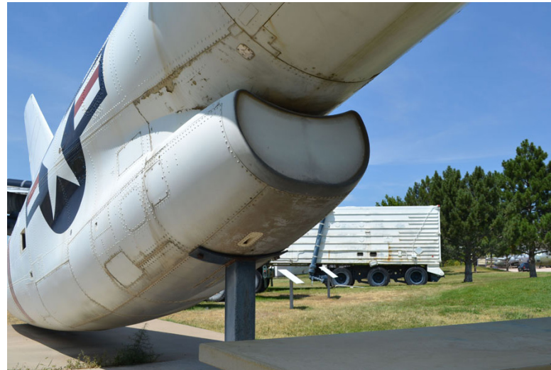
Engine intake on the Hill example. The button head rivets are quite apparent.
