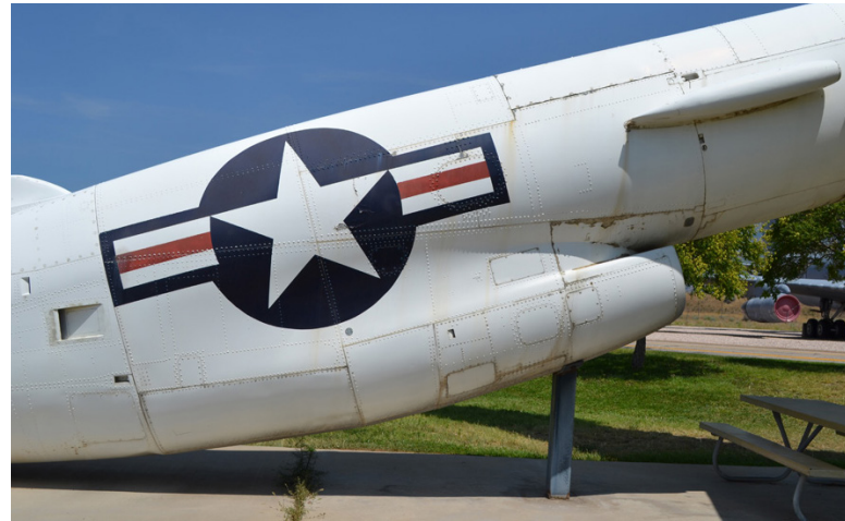
Right mid fuselage air scoop on the Hill bird.
