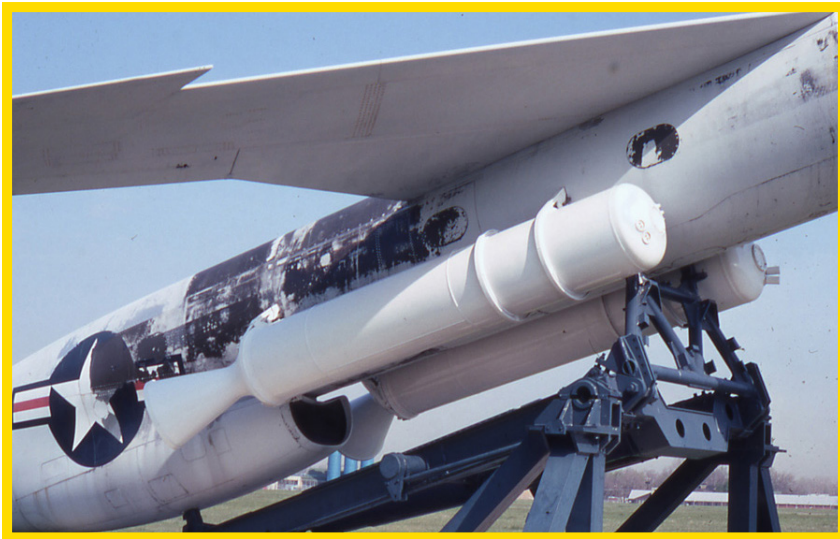
Right mid fuselage of the NMUSAF Snark with RATO booster.
