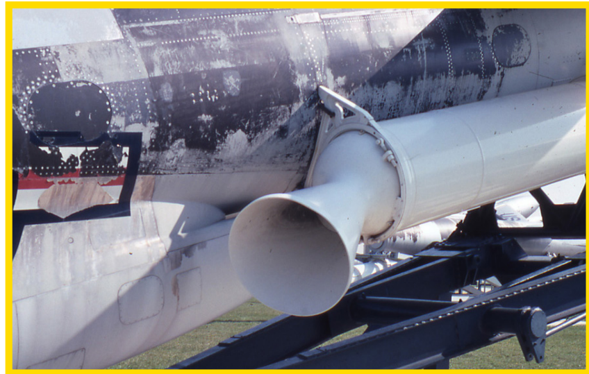
Another view of the NMUSAF Snark right side booster exhaust nozzle showing the rear support.
