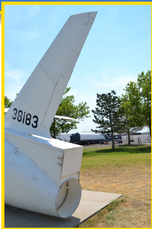
Right rear view of the fuselage tip. Note the squared off end of what appears to be a recovery parachute container above the exhaust.
