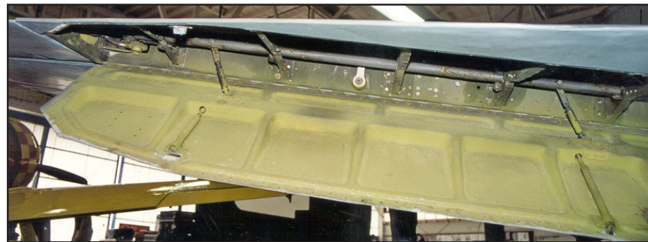
The left-wing flap interior is a yellowish green color but does not look like zinc chromate. It is the same color as shown in photo 7 of the main landing gear strut well.
