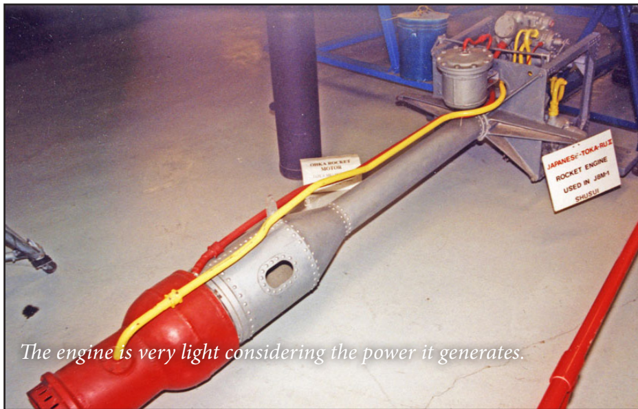
The combustion chamber appears to use regenerative cooling around the throat.
