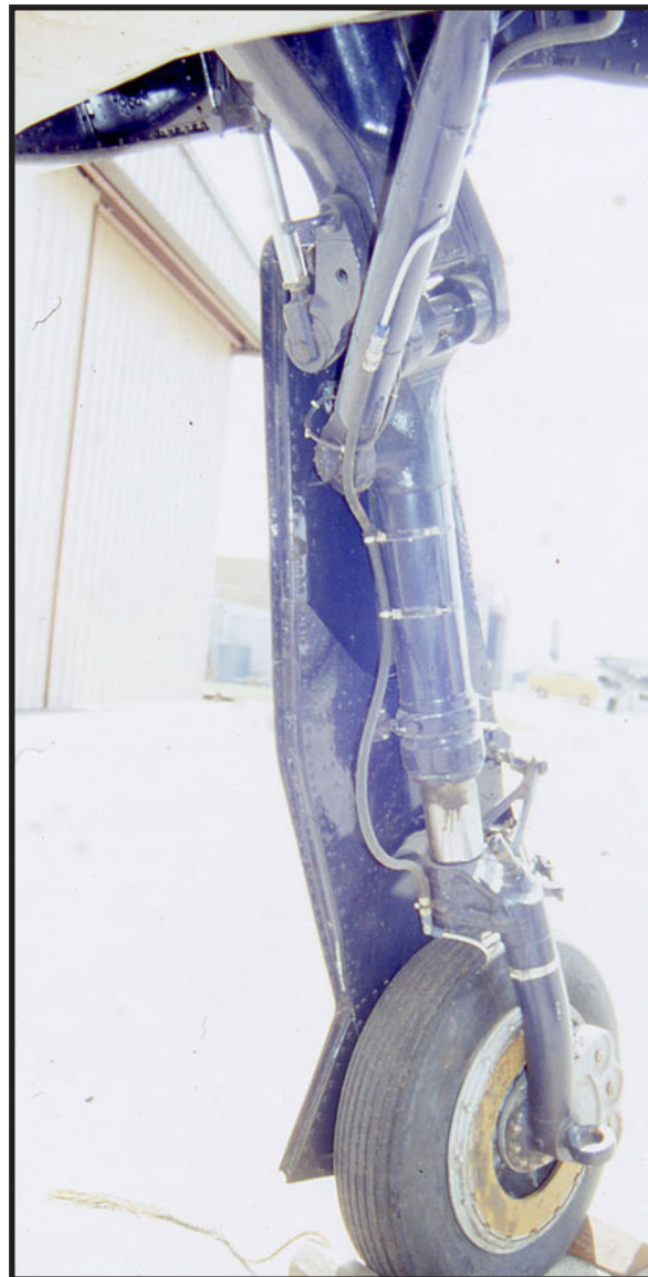
Detail shot of the Planes of Fame standard F8F. Conquest 1 was the same except the hydraulic plumbing was removed (except for the brakes) and the gear was retracted by single shot of compressed air and dropped by gravity. Therefore, the links were probably slightly different.
