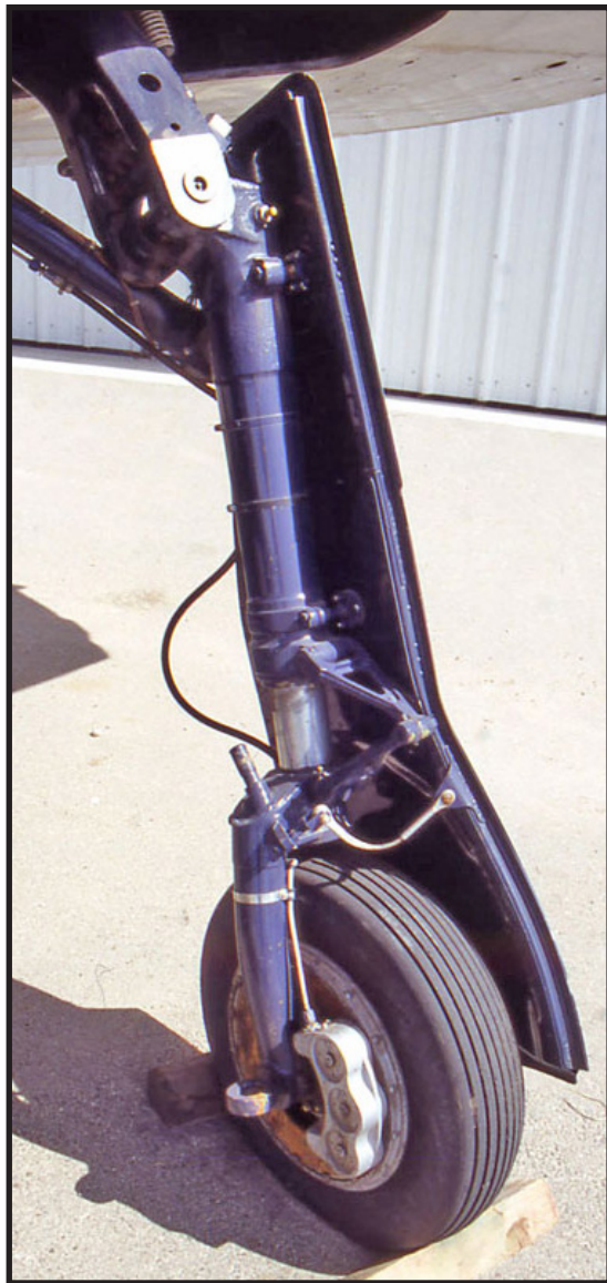
Detail shot of the left main landing gear of a standard F8F. Inboard front view. American Jet/Conquest 1 left main landing gear inboard front for comparison. Taken in 1978 at Silver Hill, MD.
