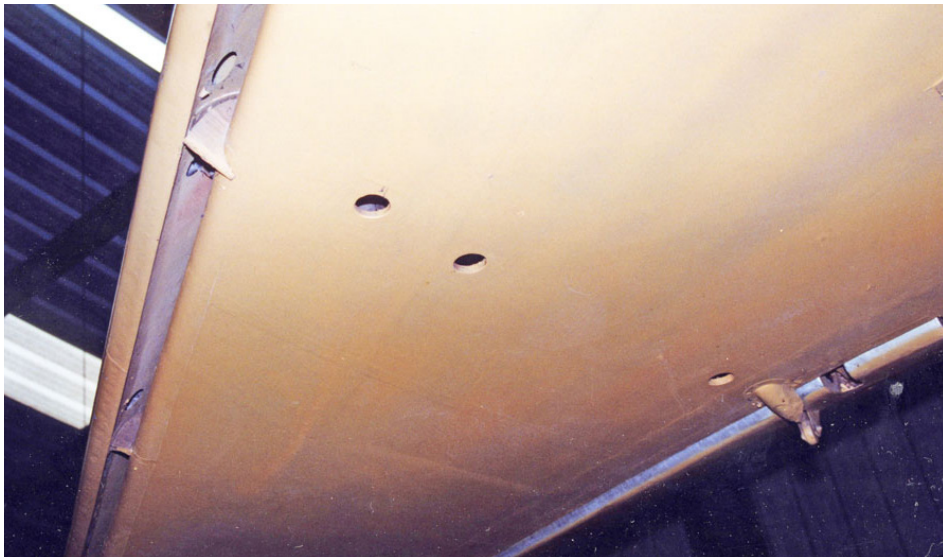
This view of the right wing lower surface shows the interior of the fixed slot.
