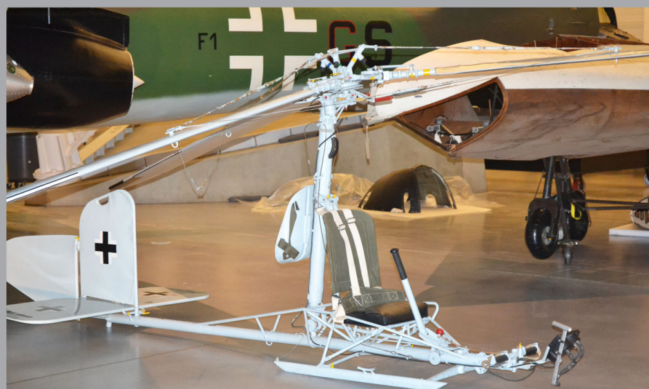
Fa 330A kite was used operationally on some submarines to provide a high look out.
