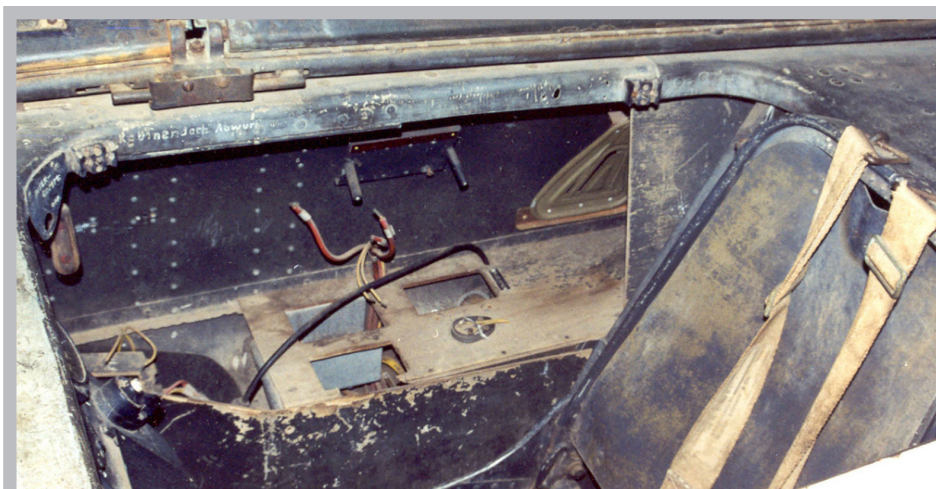
Figure 6 - Here is the starboard console of the rear seat position. Again, wood was extensively used.
