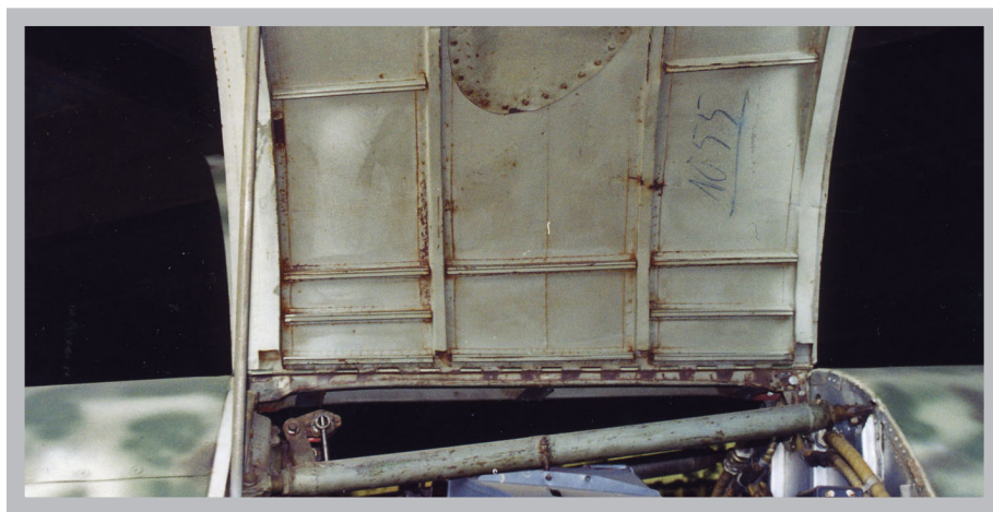
Figure 15- The gun bay cover interior was painted RLM 02 with considerable RLM 76 overspray around the edges.
