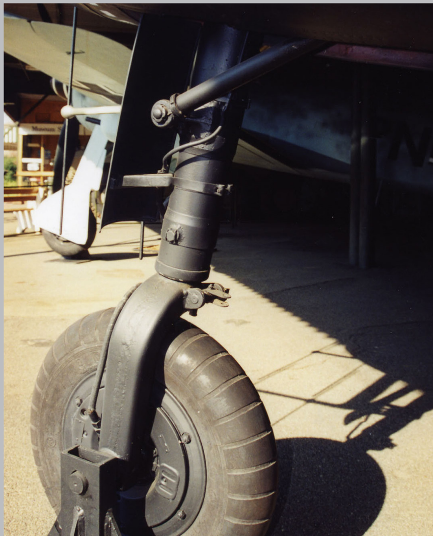
Figure 9 - The nose gear appears to have been painted black. It does not appear to be original paint. However, an analysis of period photos shows the nose gear legs of the captured B-1a/U1s were painted a very dark color, probably black RLM 22. Note the ribbed tire tread pattern.
