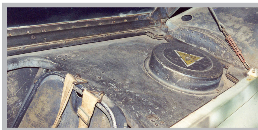
Figure 17- One of the fuel fillers was just behind the radar operator's position off set to port. The kerosene smell must have been very bad.
