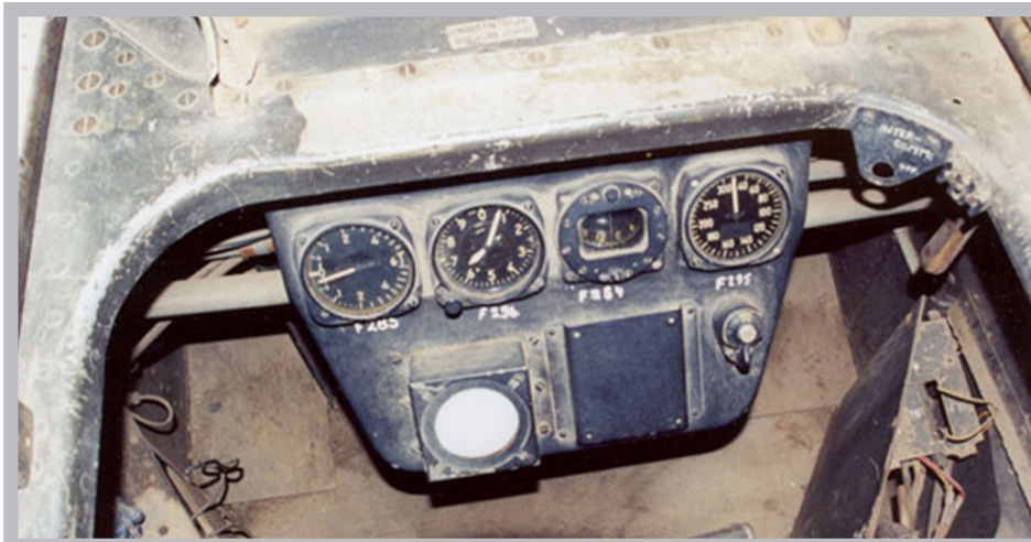
Figure 5 - The rear seat instrument panel contained the radar displays. As seen here they are British equivalents. There are subtle differences with the German instruments which can be seen on pages 178 -180 of the Kagero book "Messerschmitt Me 262 Schwalbe" by Murawski and Rys. The panel is shown in the stowed position. In operation it was rotated up to be horizontal.
