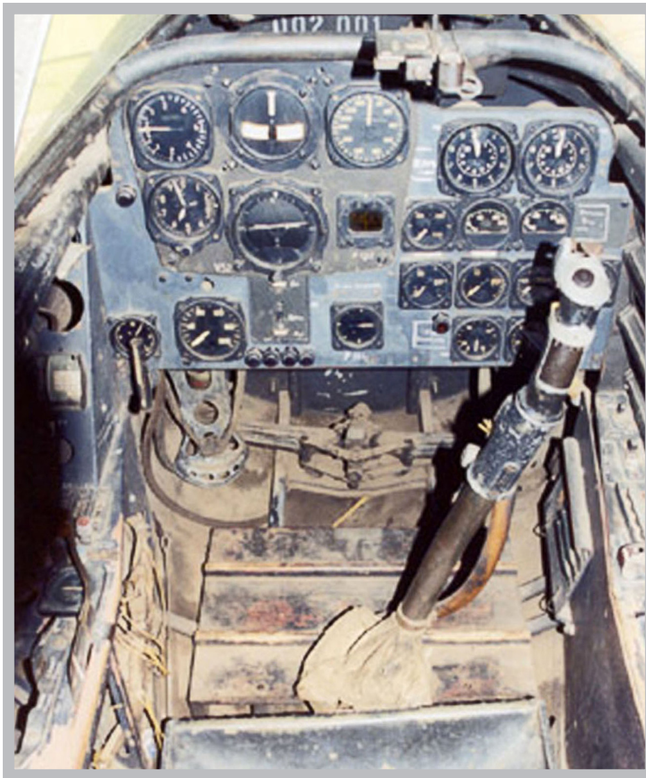
Figure 1 – The front cockpit of Red 8 looking forward. The main color is RLM 66. Instrument faces are black, and the control column boot is khaki. The flight instrument sub panel appears to be a different gray than the main instrument panel but that may be because they were manufactured by different facilities or the paint just faded or aged differently.
