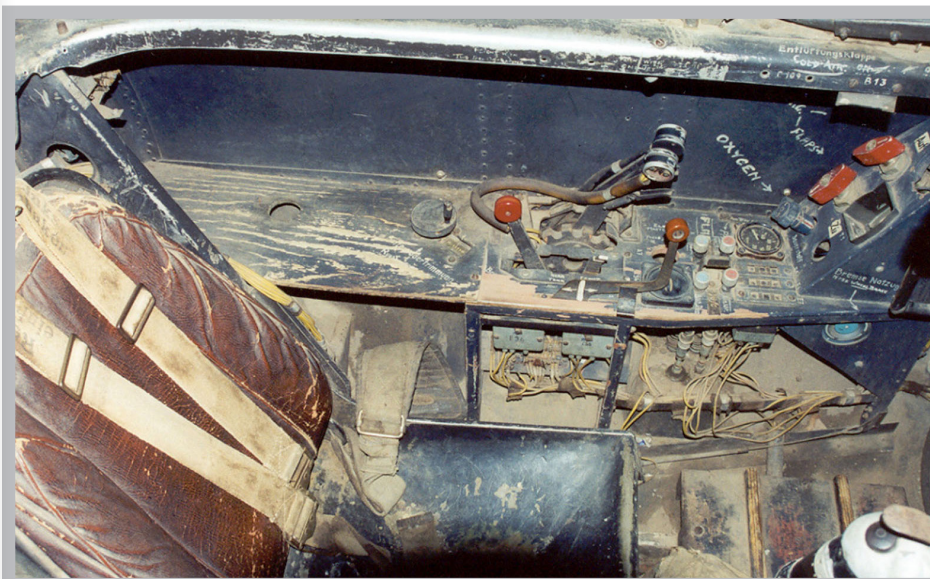
Figure 2 - The port side of the front cockpit reveals the extensive use of wood in the side consoles and floor.
