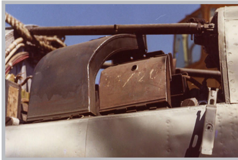
Figure 16- Starboard side view of the gun bay revealing the rusty shell ejection chutes still with some residual stenciling.
