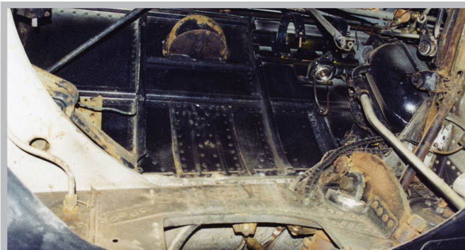
Figure 8 - The fuselage interior seen in the port main landing gear well is painted black. Various parts of the wheel well in the wing are various shades of natural metal from aluminum to steel.
