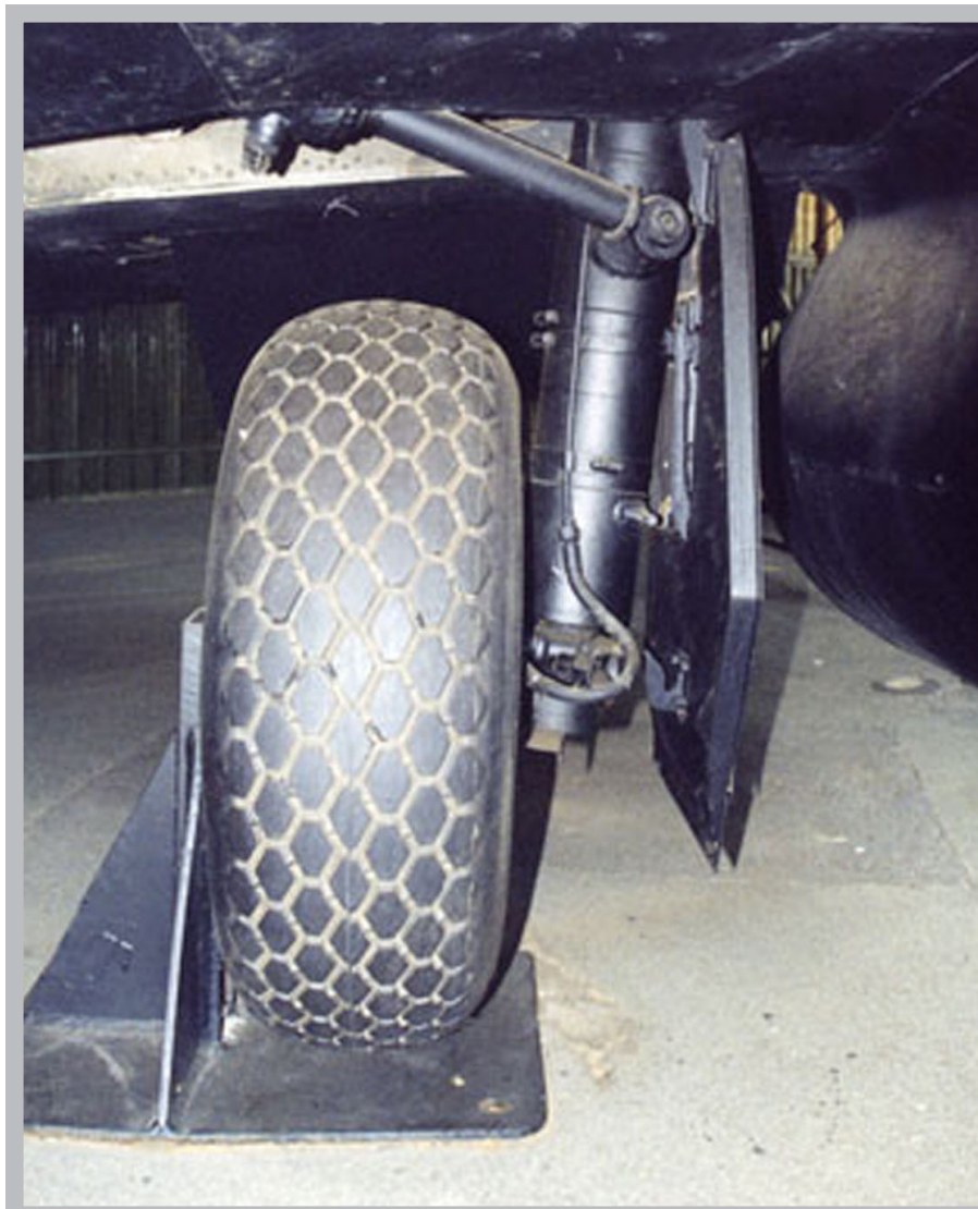
Figure 11 - The port main landing gear viewed from the front. This, also, appears to have been freshly painted black along with well covers interior. Note the tire tread pattern.
