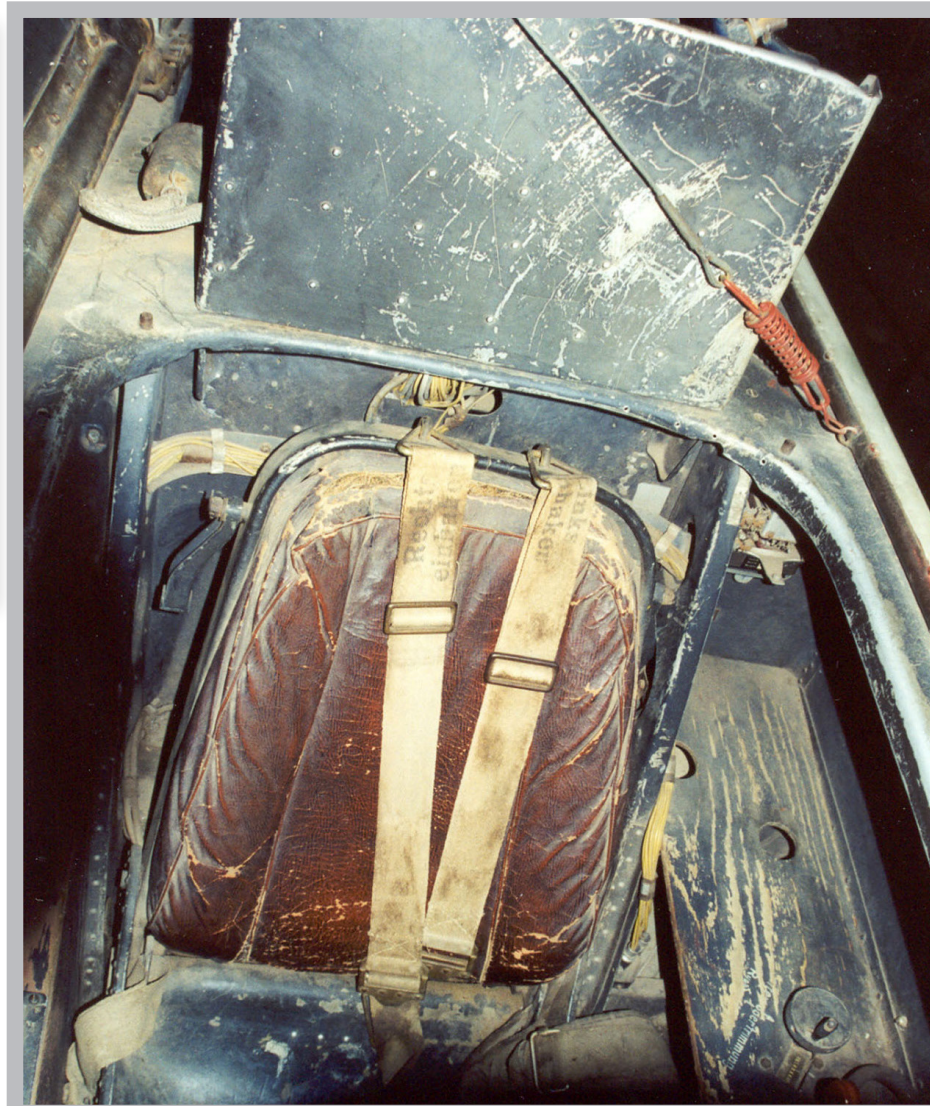
Figure 4 - The front seat has brown leather seat back cushion with khaki seat belts which are probably not the original German belts.
