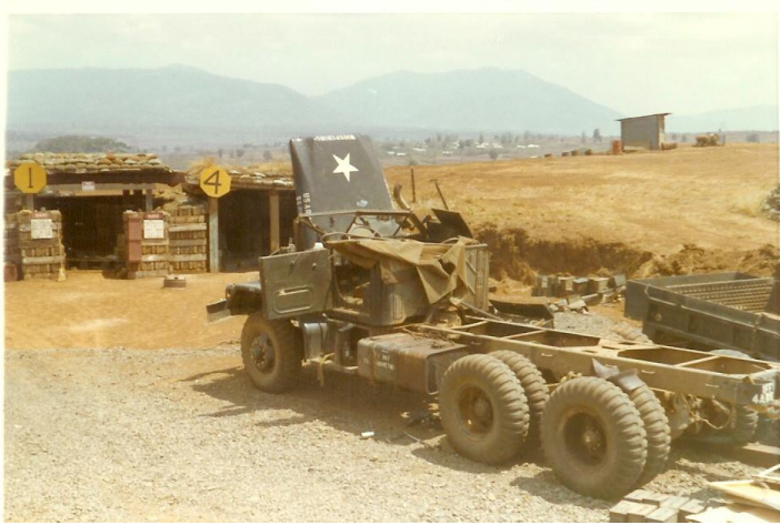
An RPG hit this Quad 50 truck at Mang Yang Pass and loosened the heavy Quad bed. The bed was removed from the chassis. If trucks were not repairable, the parts were salvaged and used to repair other trucks.
